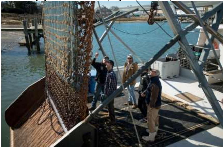
Captain Jesse Rose explains to trainees aboard F/V Midnight Our how a scallop dredge is used to harvest sea scallops offshore. Photo by Salty Broad Studios
